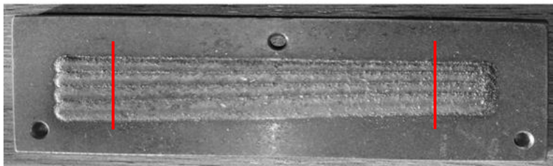
Fig. 2: A layer of deposited clad beads with the overlap percentage varying from 30% to 50%.
